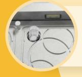
Harioculture HI incubator contains one multi-function chamber, which can monitor the droplet temperature and pH (optional) continuously without disturbing during the embryo culturing
